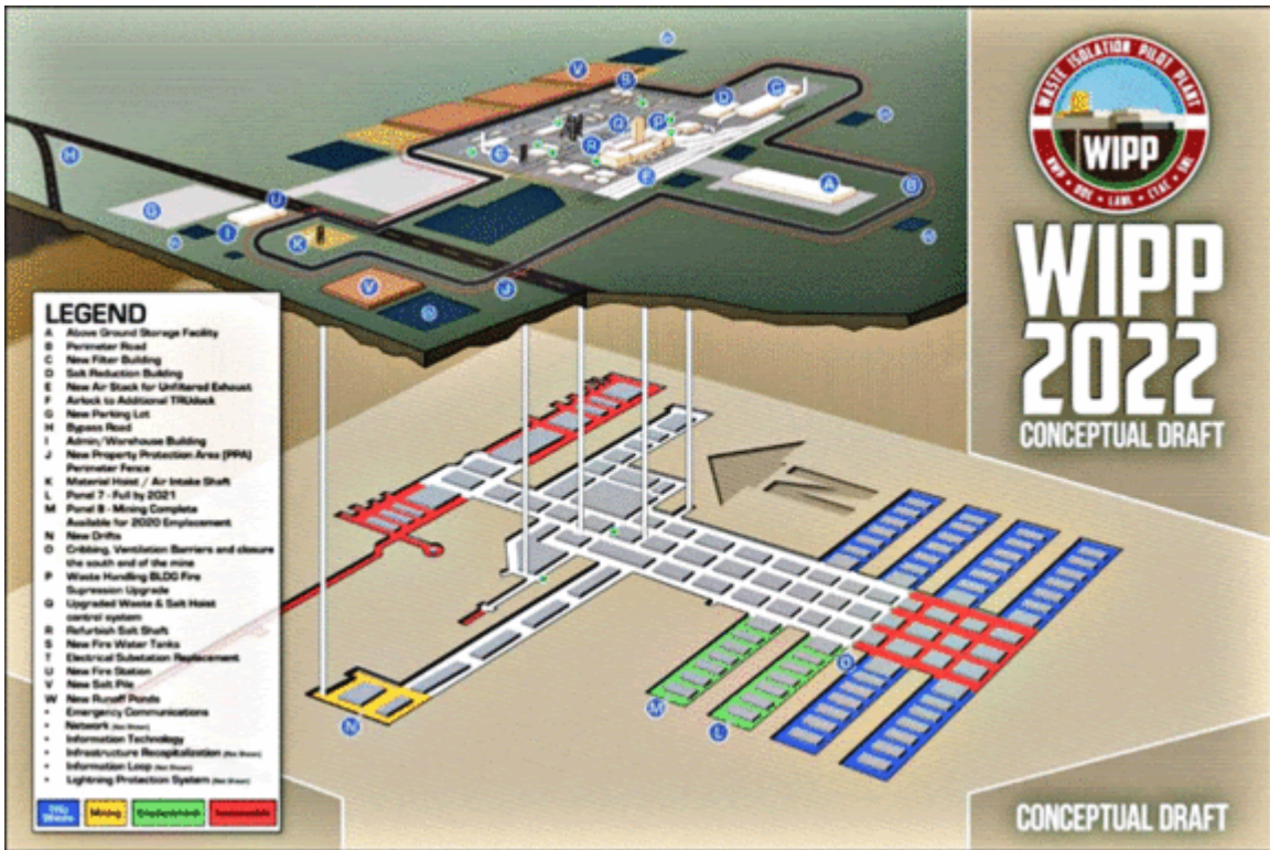
The proposed new shafts and drifts shown at K and N. The New Shaft (K) is labeled Material Hoist/Air Intake Shaft
